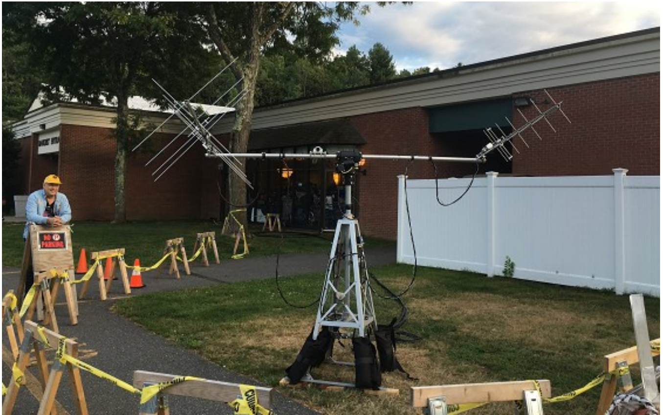
(L) Warren WAIYKF watching the satellite station automatically track 'birds' (satellites) coming within possible communication range
