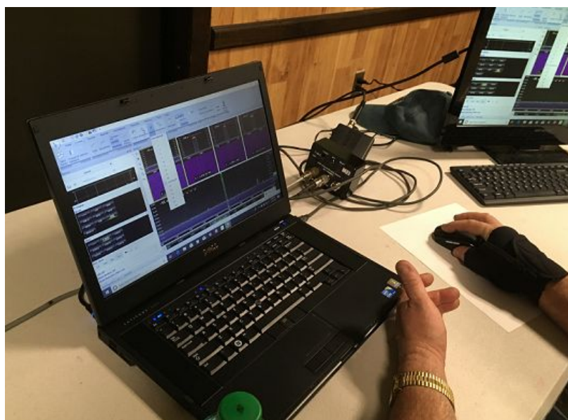
(above) The SDRPlay with its accompanying software running on Chris's laptop provides control panels and both spectrum and waterfall displays
