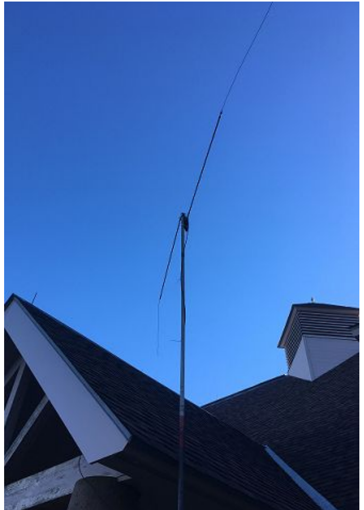
The dipole was made from 2 20M MFJ HamTenna mobile whips
