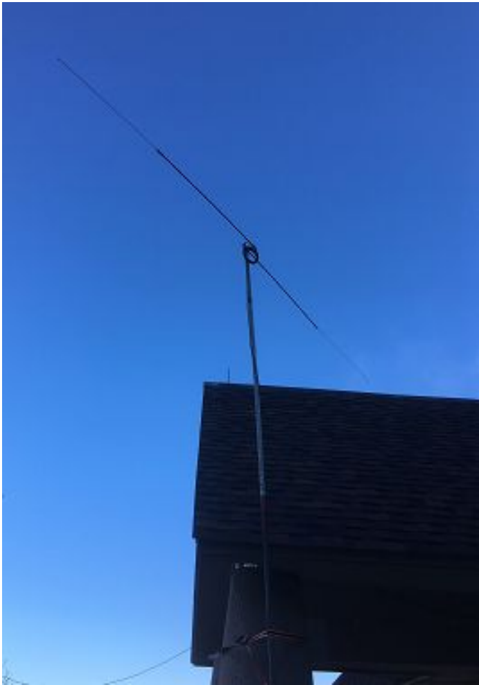
The crew assembled and raised a new 20M rotatable dipole at the visitor center this year.
