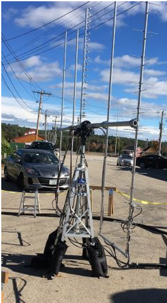
Satellite station operation by Fred AB1OC with Bob "Q" W1QWT (r) and Bob KB1FBA watching. Below shows the automated satellite tracking beam array.
