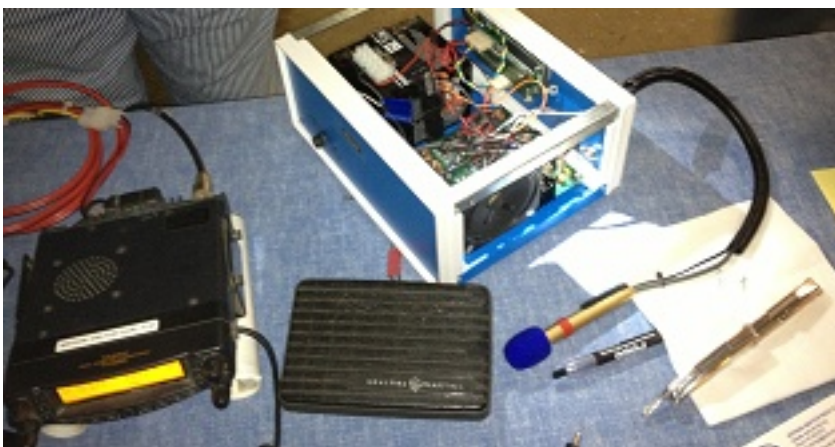
The BitX QRP transceiver next to the club's ft-8800 2m/440 rig. Several Boy Scouts made contact with club members Bill N1FRE and Mark KC1ACF through the Whitman club repeater. This helped the Scouts fulfill a requirement for their communication merit badge.
