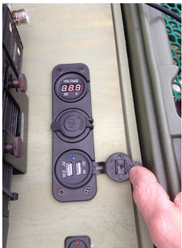
Tom also included DC voltage monitoring and USB charging ports
