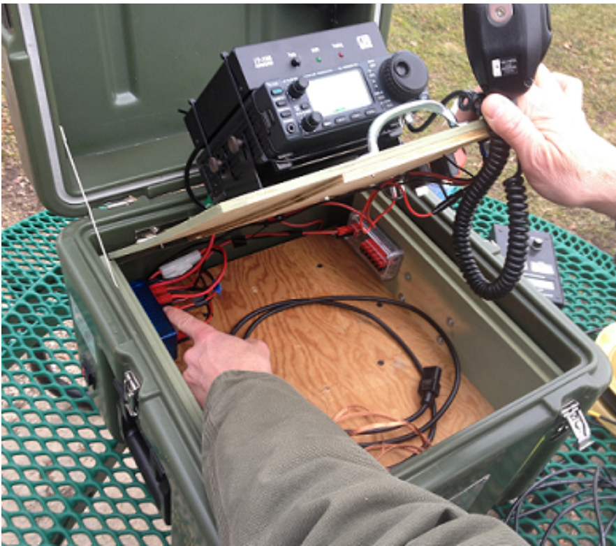
Tom WAITOM showing the power distribution wiring using Anderson PowerPole connectors.
