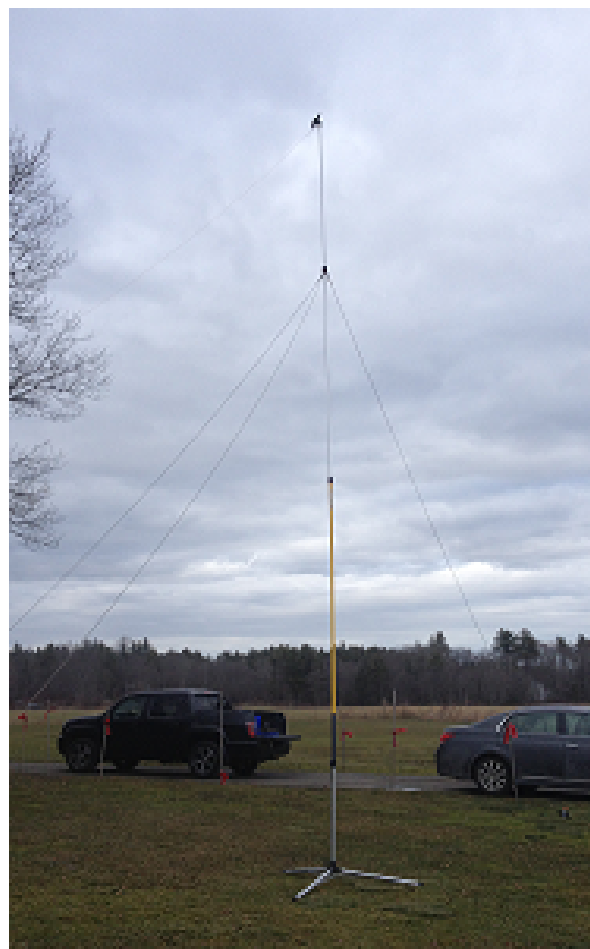
A 30' painters pole w/guy wires keeps the end of an end fed sloper up in the air
