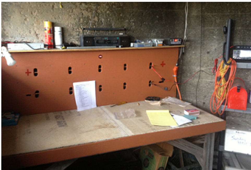
The solar powered 12volt R/C workbench provides power for the IC7300
