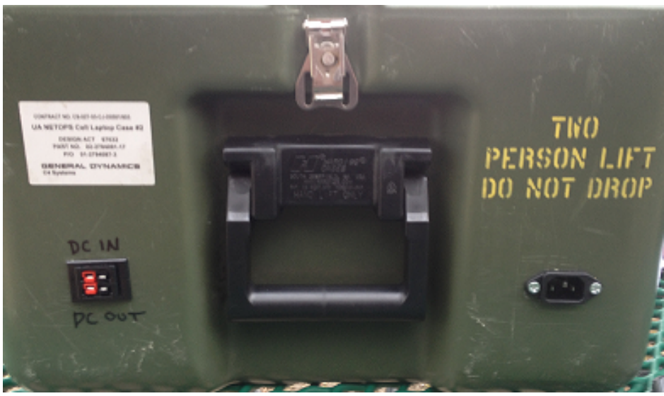
Tom's design allows for either direct 12v-dc operation or 110v a/c operation with 12v battery charging. Nice job Tom !!
