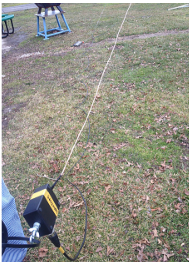
The end-fed 6-80m antenna used by Tom WAITOM
