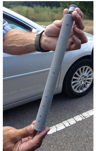
Bill NR1FD brought his completely homemade portable antenna system (similar to a buddy-pole). Bill even built his own multi-tap tuning coil from scratch
