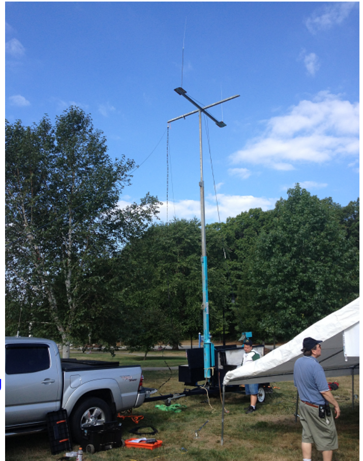
The large operating tent (top) partially assembled and (above & right) the trailer based, home fashioned tilt-over/crank-up mast system supporting mag-mount vertical antennas and the center support of a dipole.
