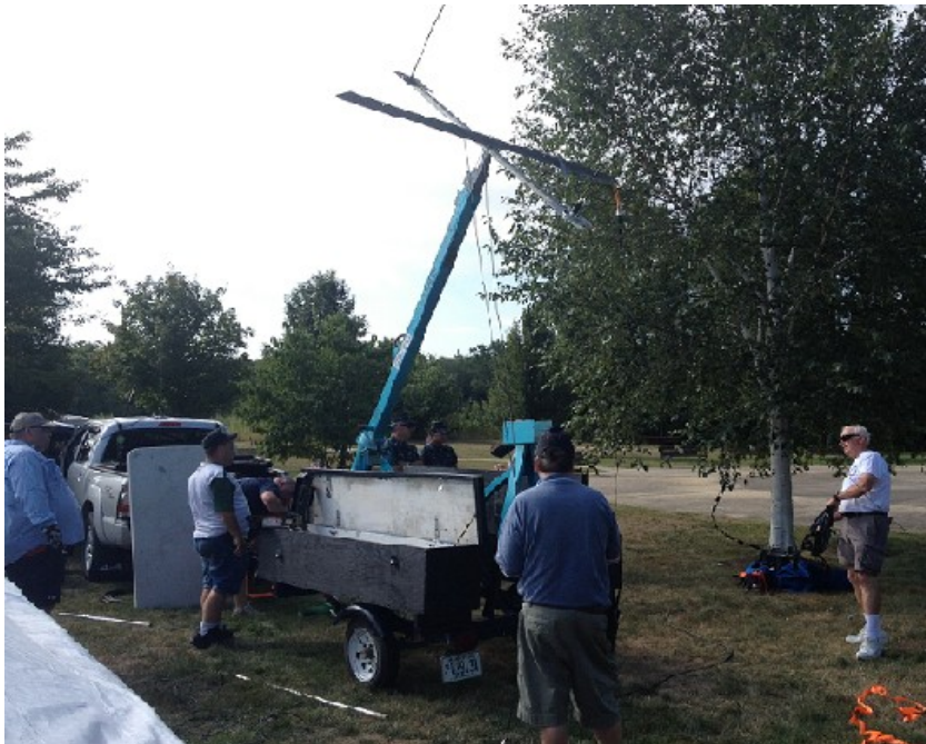
The large operating tent (top) partially assembled and (above & right) the trailer based, home fashioned tilt-over/crank-up mast system supporting mag-mount vertical antennas and the center support of a dipole.
