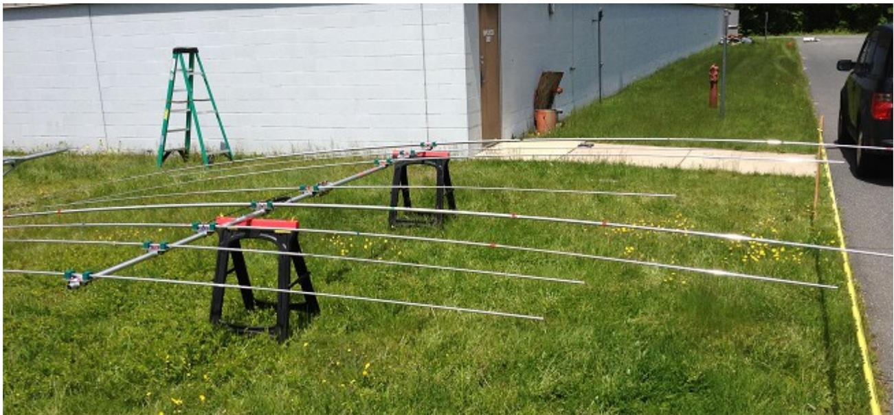
Specially designed for WRTC2014, the 20/15/10m Cycle 24 TX38 tri-bander. See <http://www.cycle-24.com/antennas/tx38-triband-yagi/> for more details.
