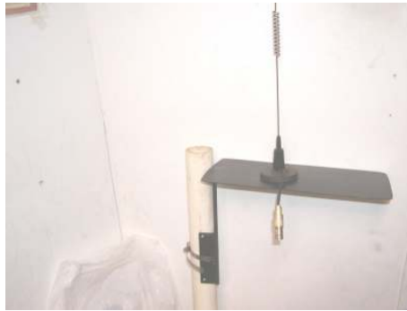
Portable antenna platform
