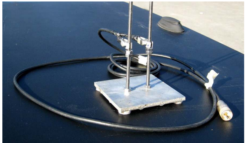
close up of alligator clip attachment located just above pre-positioned jam nuts
