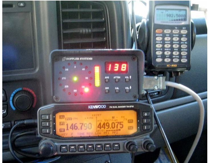
Doppler System setup for Fox Hunting
