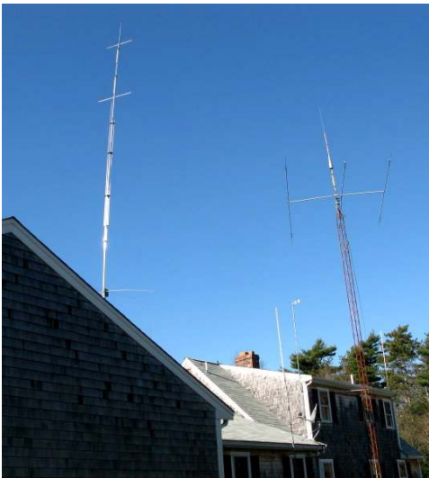
The Bruce's NI1X R-8 on the left Tower and A3WS beam on the right
