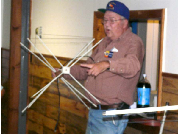
Bruce NI1X with John's WQ1L 2-Meter three element quad directional antenna
