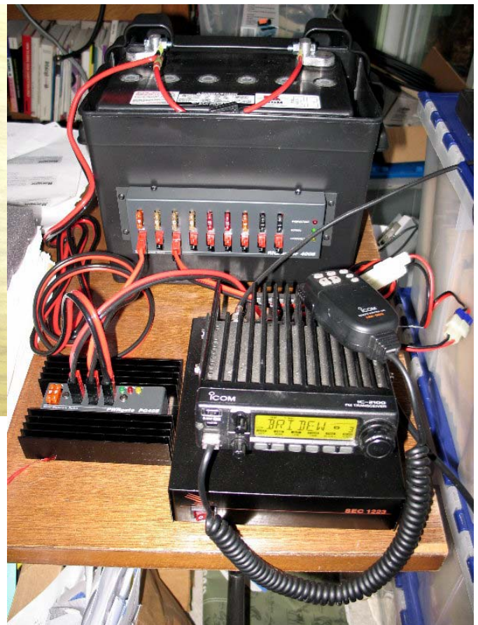
Backup battery system powering an ICOM IC-2100
