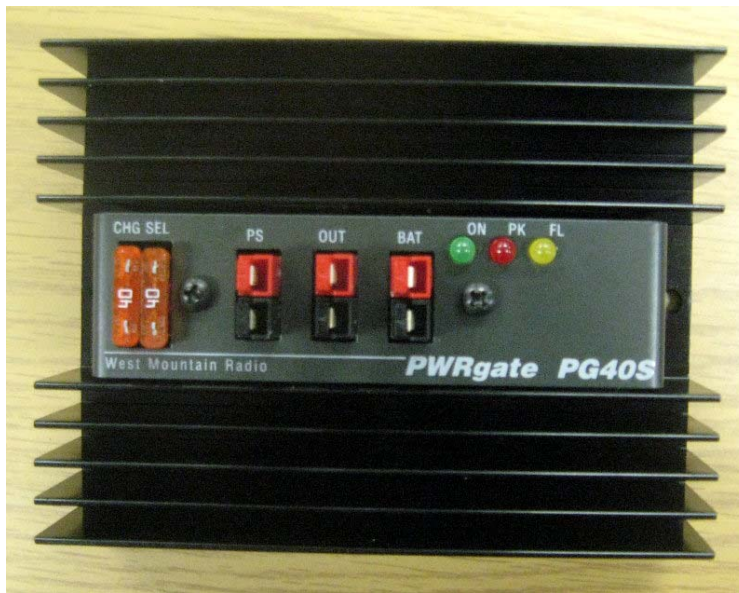
PWRgate electronic transfer switch
