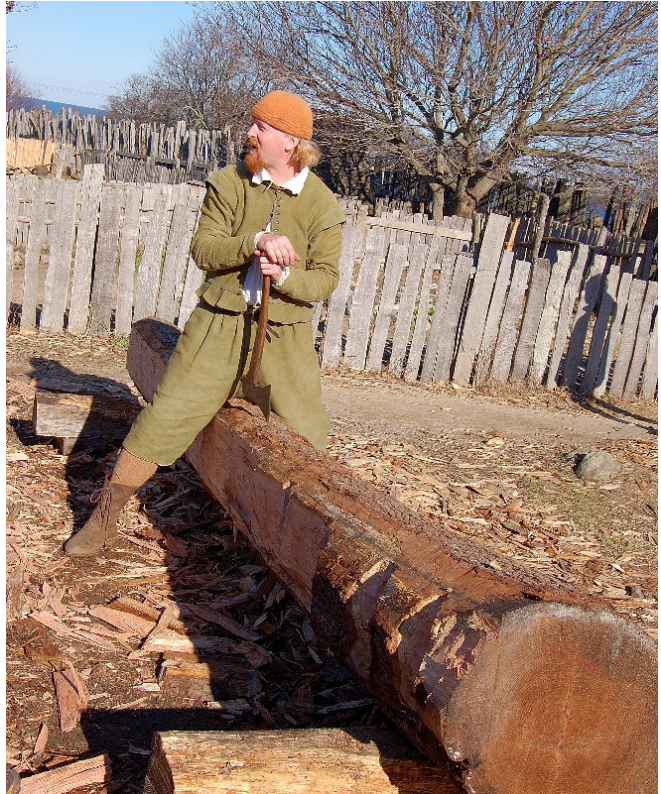
Making a beam out of a log
