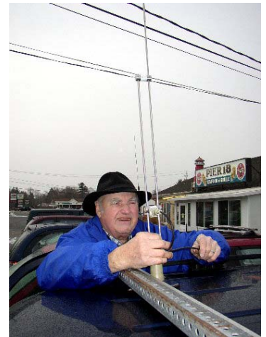
John WQ1L with his stainless steel 2-Meter J-Pole Mag-mount antenna
