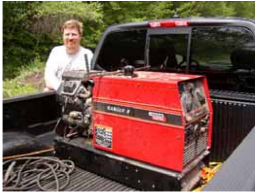
Jim Wolf N1OIU and his Lincoln Electric “Ranger 8” portable generator that is rated 8000 watts and was used for most of Field Day.
