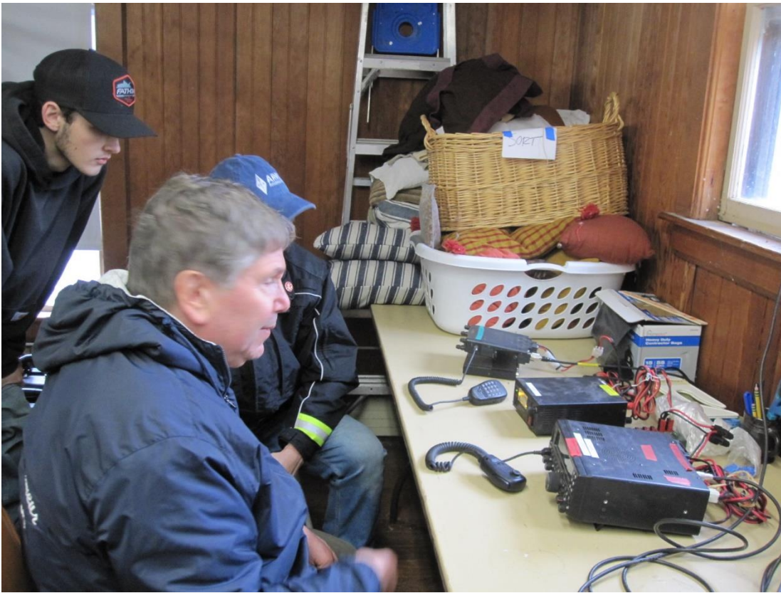
Bob WA1Q explaining the setup of the HF and 2-meter stations to Nick KC1PXJ and Lou KC1PXN. First contact after setup on HF through a pile up was Italy. We used the Yaesu FT450 with the Windom OCF dipole.
