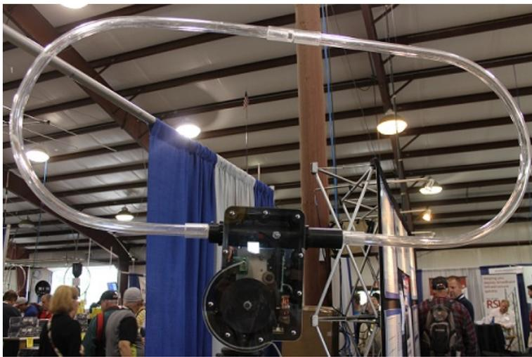
*StepIR demo model showing how the antenna radiator is re-sized for the frequency in use.*
